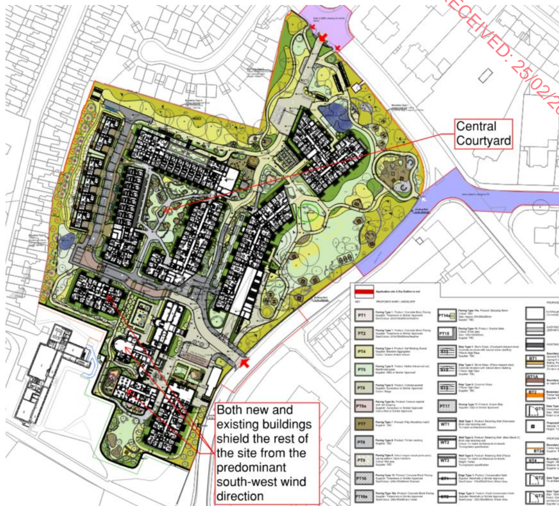
Figure 17.21: Wind Mitigation Measure – Apartment Block Arrangement
