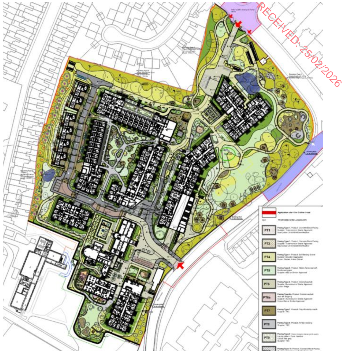
Figure 17.23: Wind Mitigation Measure – Landscaping Design (Ground Level)
