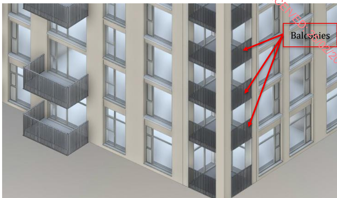
Figure 17.22: Wind Mitigation Measure – Block A1 Inset Balconies
